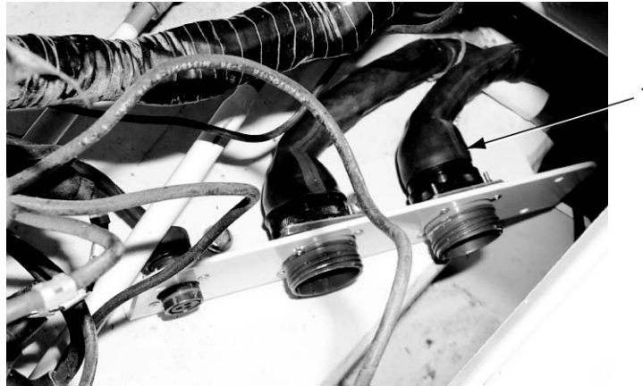
Figure 5-5. Initial Placement of Lower Cable Assembly W3
