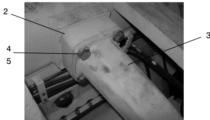
Figure B-6. Spacer Block Installed
