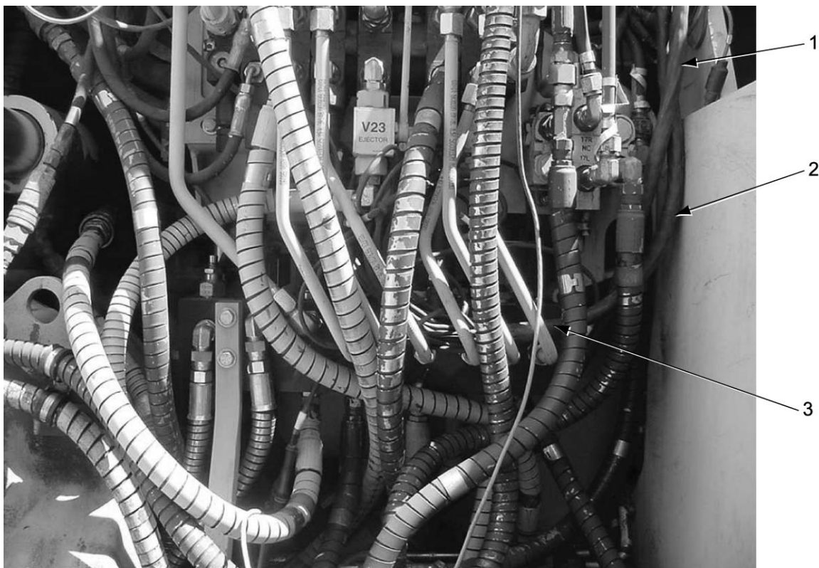
Figure 5-12. Upper Cable Assembly W2 Routing
