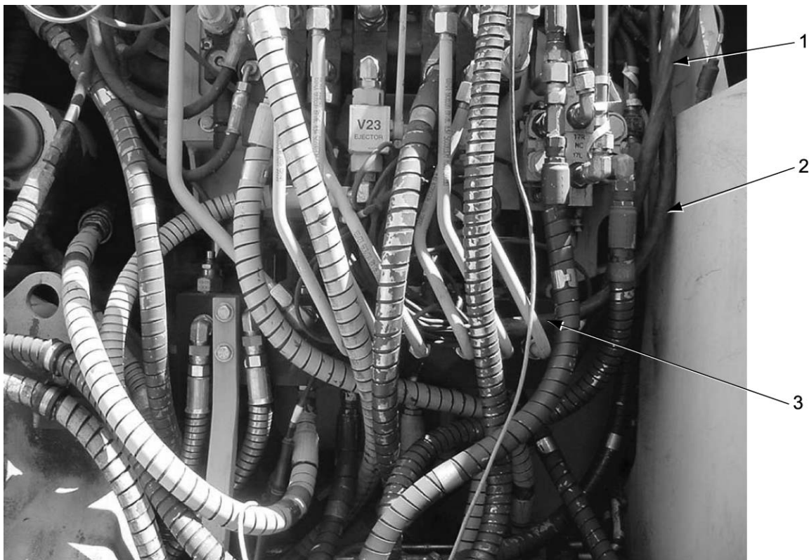
Figure 5-12. Upper Cable Assembly W2 Routing
