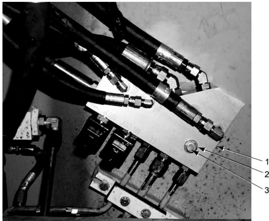
Figure 4-10. Installation of New Forward Right Manifold Assembly
