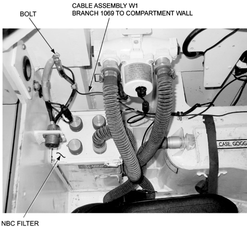
Figure 5-11. Routing Cable Assembly W1 Branch 1069 to Compartment Wall
